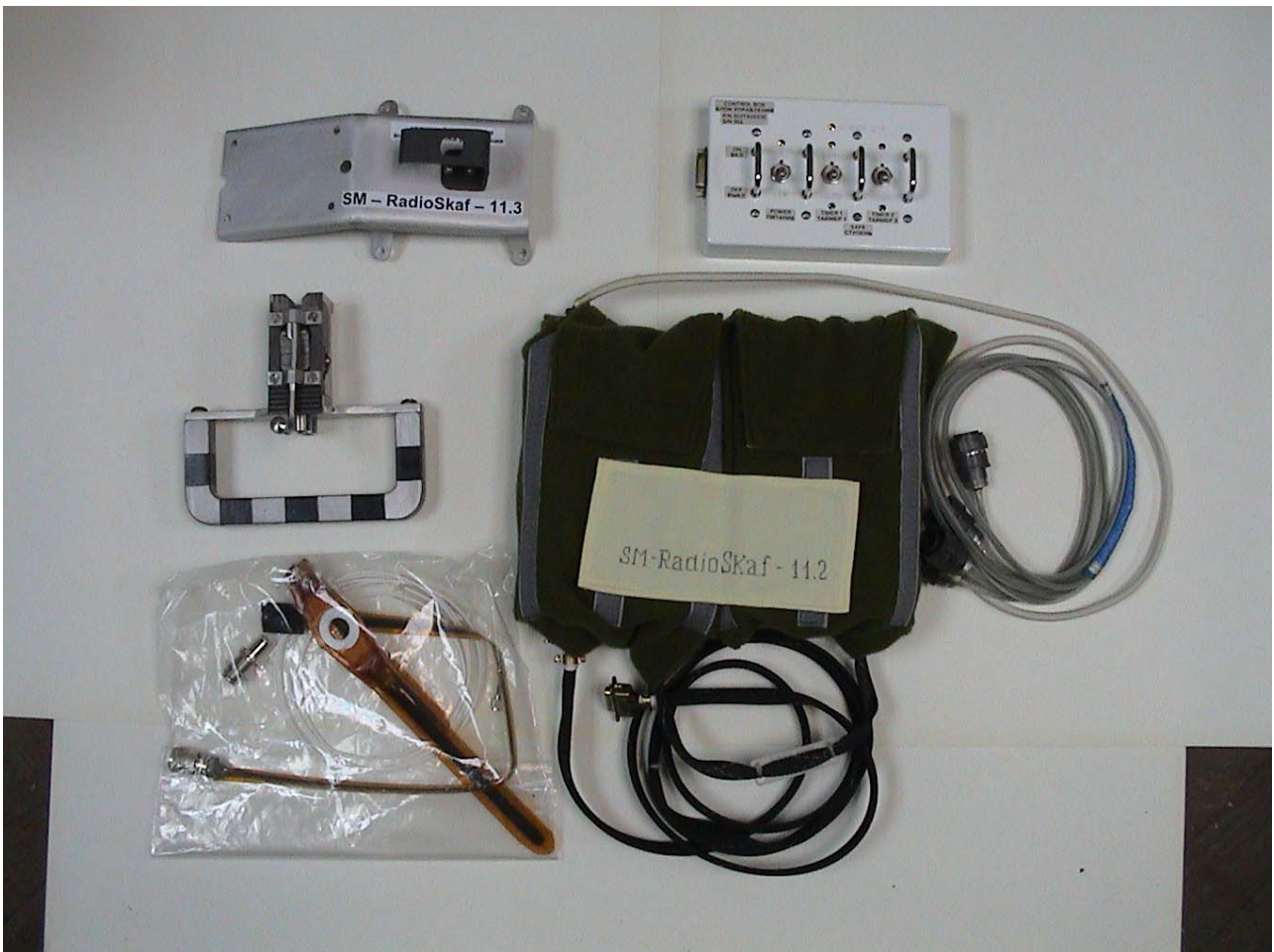
Suitsat Hardware (Transmitter and Digitaltalker/Microcontroller Box inside Fabric Container) Figure 6
