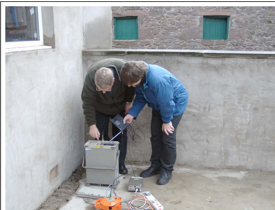
Fig. 2. First experiments in the yard of premises A. The spectrum analyser and pre-amp for the current clamp can be seen, together with the domestic portable radio (only being used as a pointer here!).
