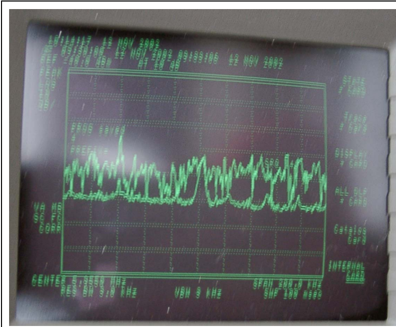
Fig. 5. Spectra obtaining using loop antenna, for comparison with the current-clamp measurement of Fig. 3. The noise floor was higher than expected, but there is still a clear distinction between modem on and off conditions.
