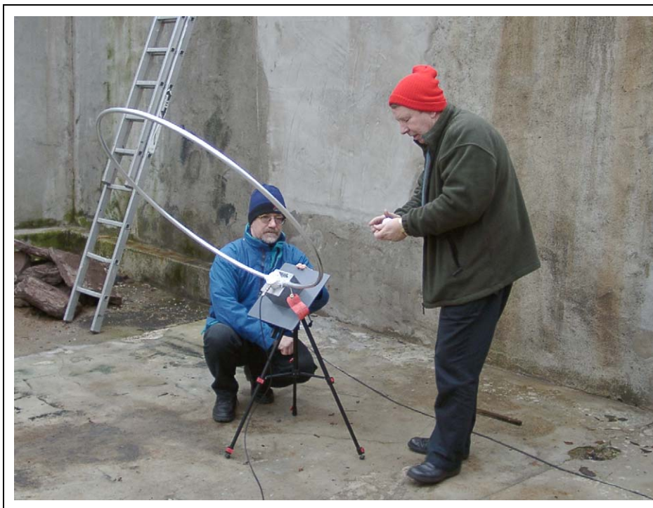
Fig 4. Adjusting the loop position for maximum coupling to the extension cable (on the ground), in the yard of Premises A.
