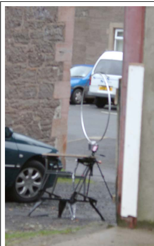
Fig. 6. The loop positioned on its tripod in order to measure emissions from the lamp-post (which is not itself visible in this view). The view is from the yard of premises A, with the house itself on the right. The house on the left is the start of the adjoining terrace on the other side of the access drive.
