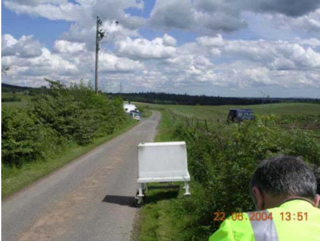
Figure 11 Loop Antenna 30 metres from the downstream launch point (Span 1)
