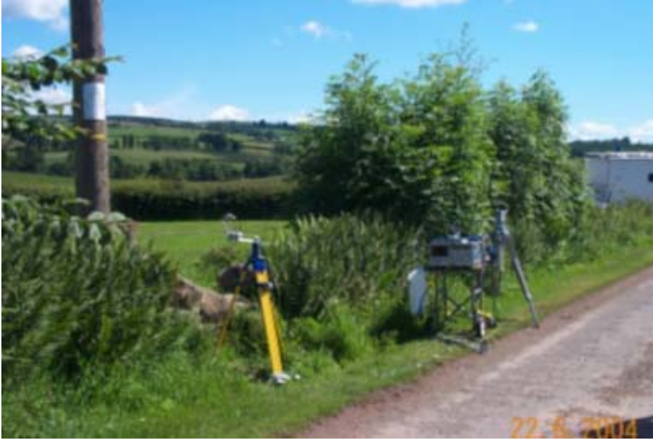
Figure 4 Measuring Equipment by the Downstream injection Point
