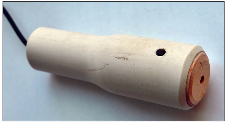
Figure 6: Microphone for the QMX+ transceiver made from a scrap piece of PVC pipe. The microphone element is glued on the inside back of the thin plywood end cap. A second end cap seals the back end of the pipe. The plunger of the push-to-talk push button protrudes through the side wall of the pipe while the switch itself is held firmly in place with a wooden wedge inside the pipe.
