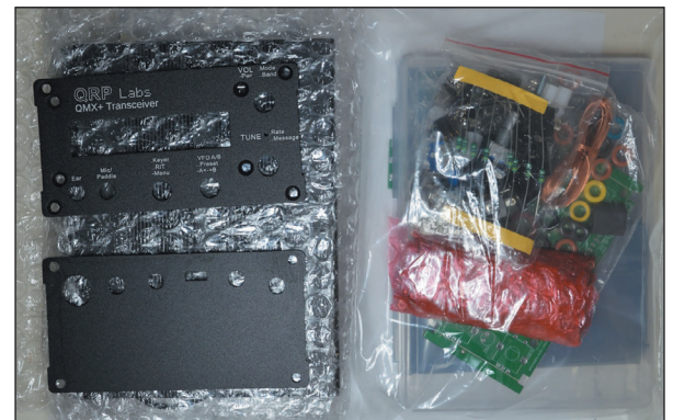
Figure 3: QMX+ kit components. In the photo the circuit boards are packed under the front and back panels on the left and other components are in the plastic bag shown on the right.
