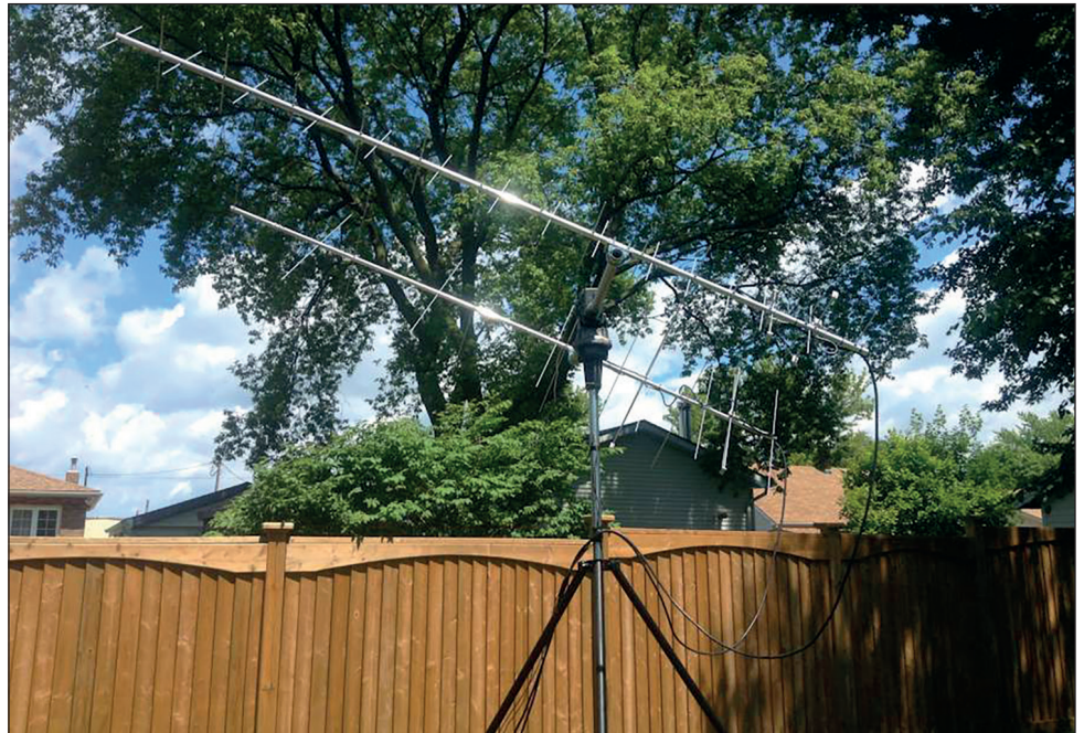
I use a pair of "long boom" M2 crossed Yagi antennas and about 8 metres of Times LMR-400 feedline. This arrangement precludes the need for mast-mounted preamps, as the internal preamplifier in my TS-2000 radio has proven to be sufficient. (Courtesy: VA3KSF)
