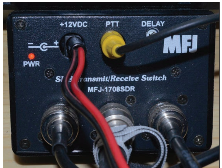
Figure 3: The MFJ-1708SDR switch that allows the safe connection of an antenna to both an SDR receiver and a transceiver. The antenna is connected to the coax connector in the centre, the transceiver and the SDR receiver on the other two. There is also an MFJ-1708B-SDRS model on which the SDR connection is an SMA instead of an SO-239. This change of connectors would prevent confusion between connections.
