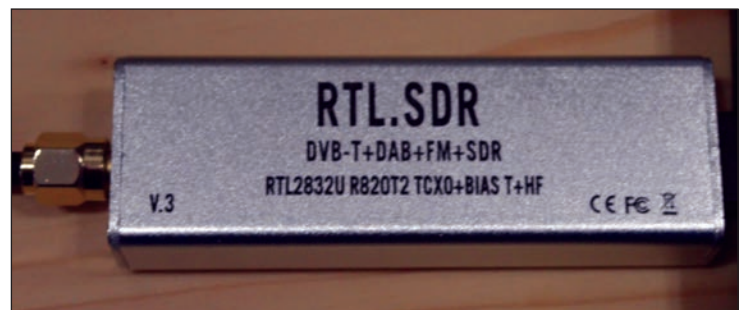
Figure 4: The RTL SDR dongle used by VY1GP.
