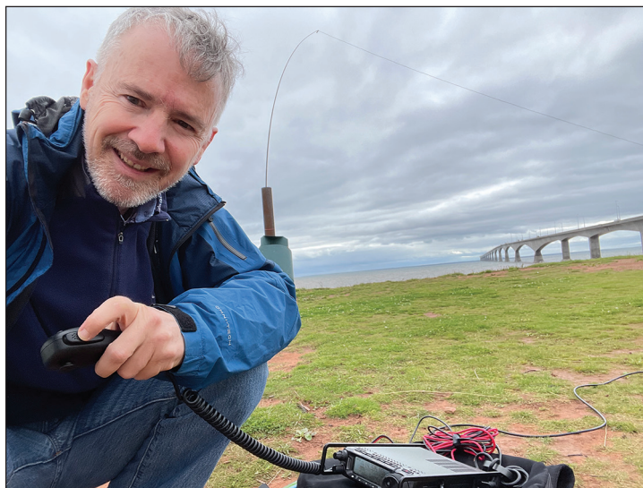
Robbie Morrison, VE7NB, conducts his POTA activation from Marine Rail Park (VE-5775) near the Confederation Bridge on Prince Edward Island. His carry-on fly-away kit is comprised of a Yaesu FT-891, 20m end-fed half-wave (EFHW) antenna, 50-foot coax, and a 12AH Bioenno battery.
