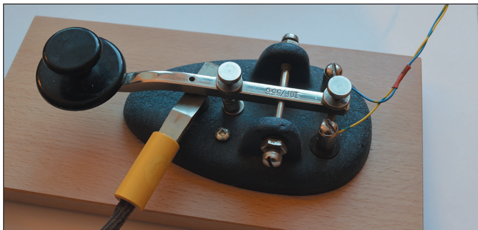
Figure 8: A "Wilson" straight key with a wedge inserted between its contacts.
