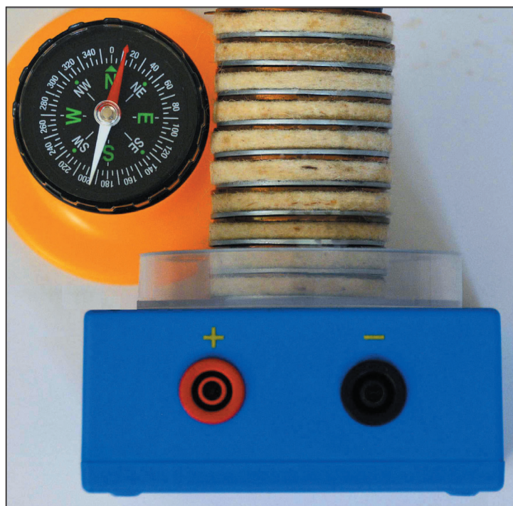
Figure 8: The “Romagnosi Effect”. This Eisco (10-cell, 10-volt) voltaic/galvanic electrochemical battery is operating in open-circuit mode; therefore no external electric current can flow. Yet “something” is pulling the compass needle – first aligned to magnetic north – north-north-east. This battery uses pure copper and zinc discs (both non-magnetic) and felt washers mounted on a plastic spindle and base. More importantly, there was no magnetic needle deviation until after the felt washers were dry-soaked in acetic acid (vinegar). This is definitely not a static electricity effect!
