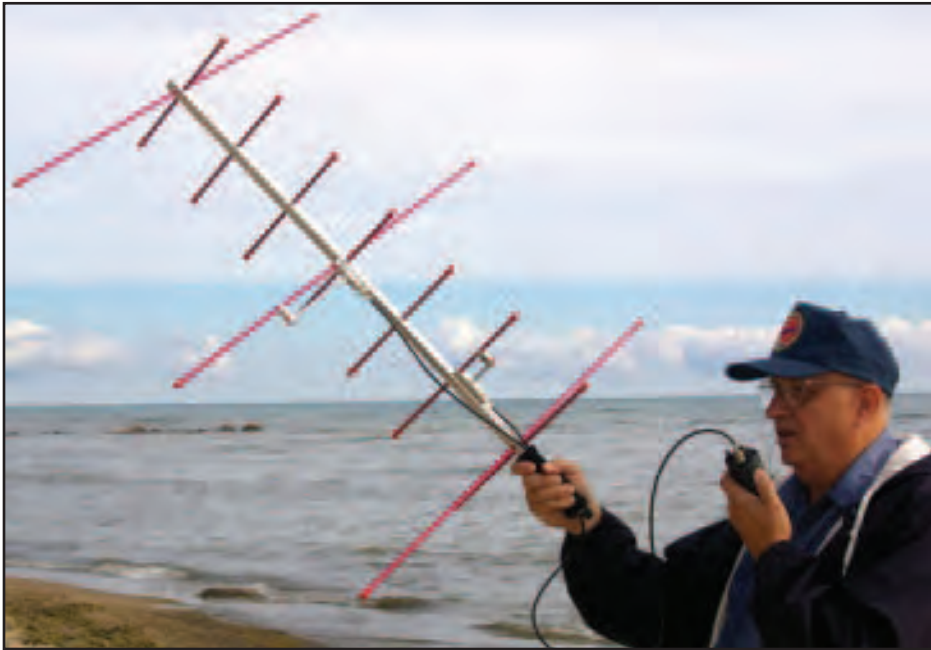
Keith Baker, VA3KSF/KB1SF, our new columnist, uses a Kenwood TH-78A dualband HT and a lightweight Arrow Antenna (Model 146/437-10) to make a contact through an AMSAT Amateur Radio satellite from the shores of Lake Huron. When used with a 5 watt, full-duplex handheld in an open location free of foliage, such as a beach or a field, the antenna provides enough uplink and downlink gain to successfully work the FM birds, even on passes close to the horizon. (VA3OGF Photo)
