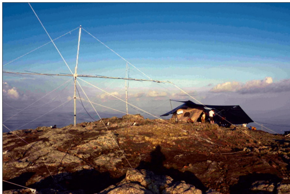
The Malpelo Island 6m operating position, with 8-element yagi, atop a 900-foot rock. (photo courtesy of the HK0NA website at http://hk0na.com/ )
