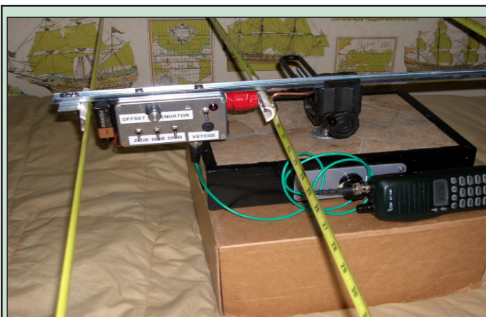
Figure 4: Fox Antenna with Cast Aluminum Box and Metal Boom
