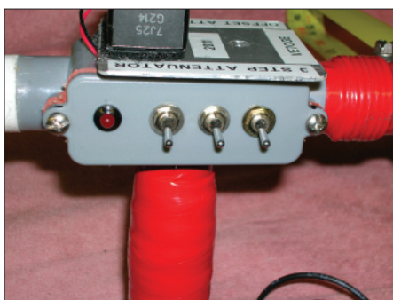
Figure 2: Basic Fox Antenna with a Three-Step Attenuator and an Offset Attenuator.
