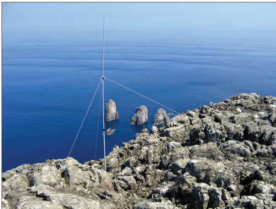
The "Three Musketeers and D'Artagnan" rocks with antenna support (looks like a vertical but actually supports one end of a wire antenna).
