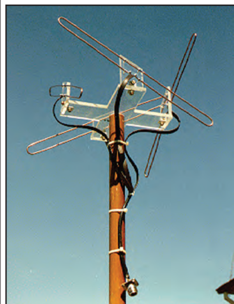
The Lindenblad antenna is yet another, relatively easy to build omnidirectional antenna suitable for satellite work. (Courtesy: AMSAT)
