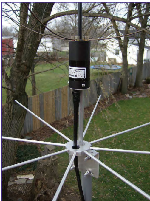
Here's a partial view of the phasing coil and ground plane of the author's 2m, M2 "Eggbeater" antenna. Note that the ground plane radials are offset by about 1/2 wavelength (10.5 inches) from the top of the phasing coil and driven elements. (Courtesy: VA3KSF)
