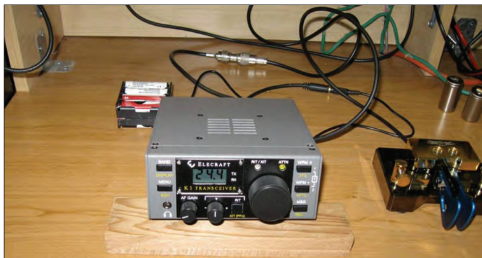
“Here is the newly-built Elecraft K1 shown just after making a contact with LY2XW (Vygis in Lithuania) Saturday morning. The output power at this end was 3 watts on 14.0244 MHz using Morse. The 12 volt supply was a group of eight AA alkaline cells housed in a pair of 4-cell holders purchased from The Source (ex Radio Shack). The Morse paddles are one of my Begali iambic paddles. The LY2XW station had a very strong signal (S9) and he gave me a signal report of 589.” — John Noakes, VE7NI
