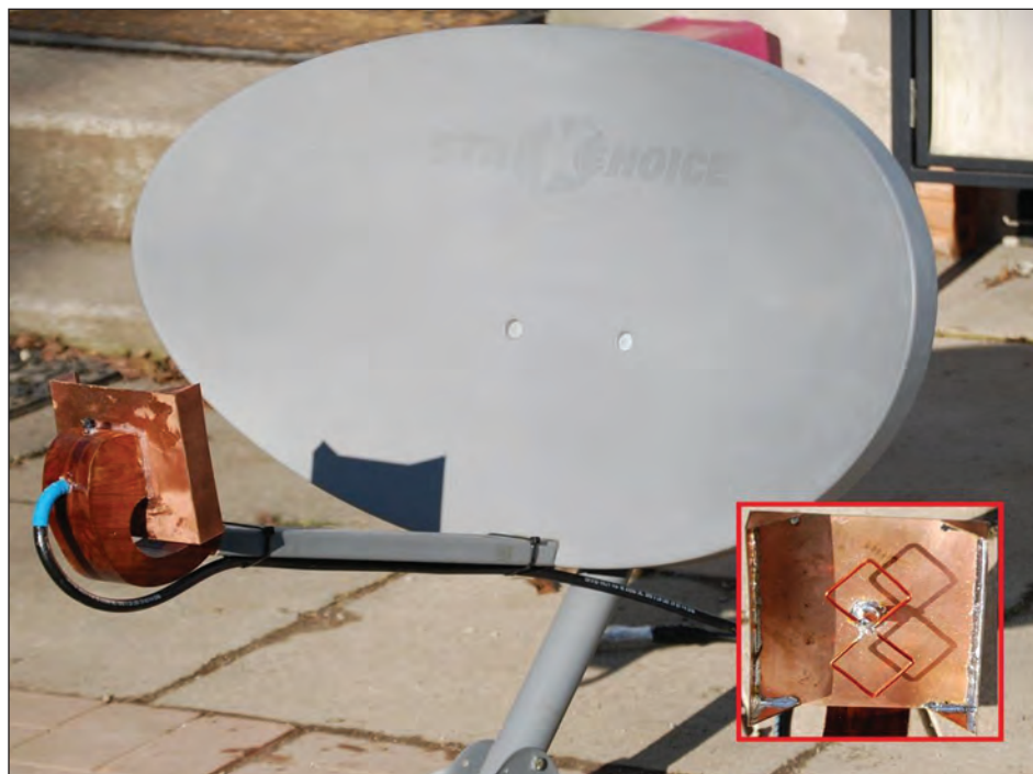
An old satellite dish refurbished for use on the MESH system; Image courtesy of Brad Fowles, VE3HII.
