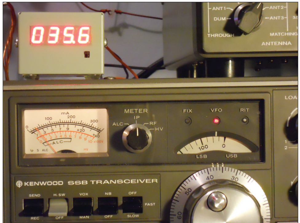
Figure 1: The digital dial on top of my TS-520S transceiver. The analog dial shows .036 MHz. The digital dial gives a more precise .0356 MHz.
