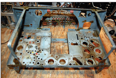
The original chassis with all components removed
