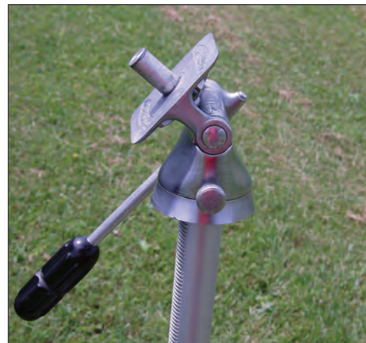
The short stub screwed into the tripod head. The angle of maximum elevation of the upcoming satellite pass is set with the tripod's elevation control. Here it's set to about 45 degrees.
