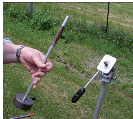
The basic Gizmo with the counterweight, main shaft, plumber's tee and bushings installed. Note the drill stop between the tee and the weight. This addition is not necessary but Art found it handy so that the shaft didn't slide in the tee when attached to the antenna. Also note the short stub attached to the tripod.
