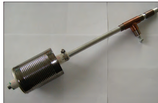
A "soup can" counterweight made from a split PVC pipe and a stainless steel hose clamp. The can is filled with cement and mounted on the Gizmo.
