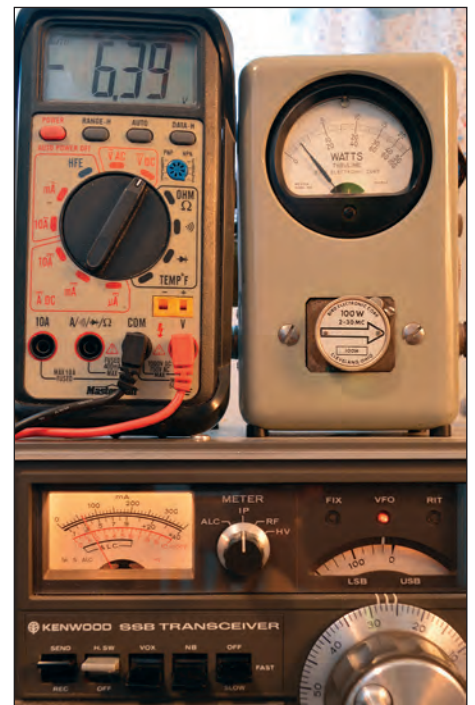
Figure 4: QRP power at about -6 volts ALC.
