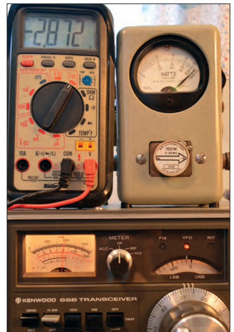
Figure 3: Full power output at about -3 volts on the ALC terminal.
