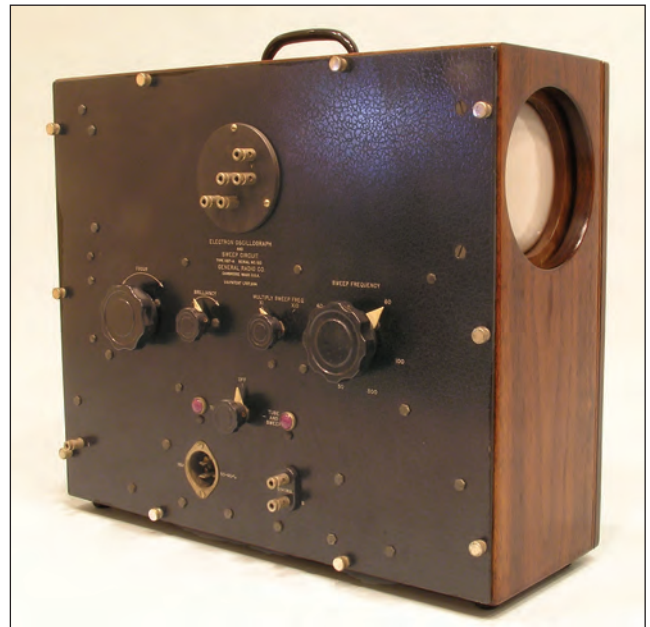
The Type 687 Oscilloscope. With only the tube and horizontal sweep electronics, the user supplied any vertical gain. Courtesy of the IET Labs website (see the text for the URL).
