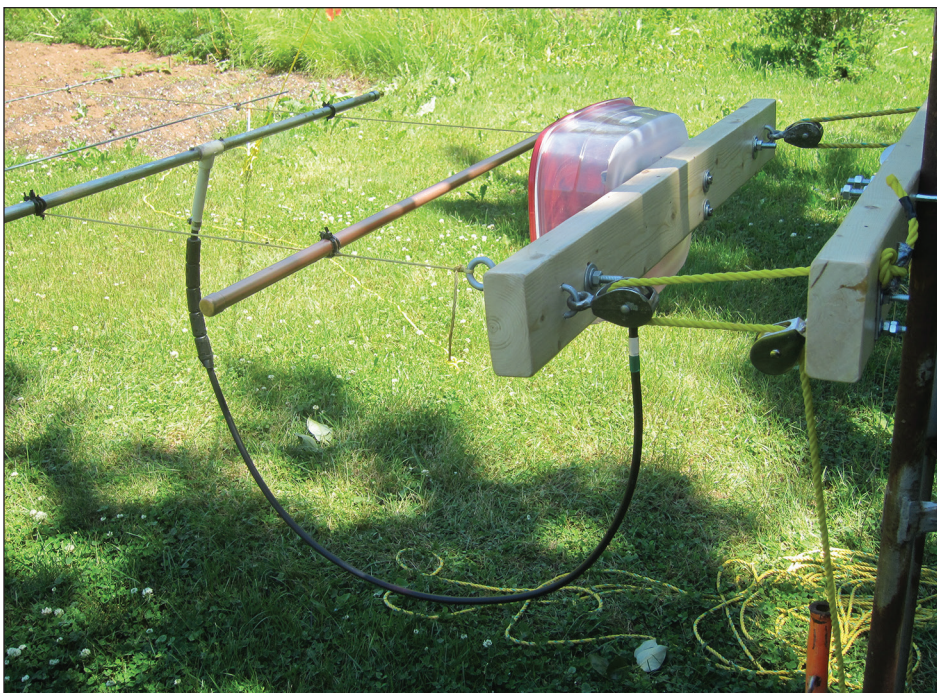
Figure 3: Feedpoint of just-completed yagi. The pulleys provide 2:1 mechanical advantage for tensioning. The plastic box contains the coaxial transmit-receive relay and GaAsFET receive preamplifier. Long eye-bolts through the pulley block allow adjustment of the Kevlar boom-to-element angle to 90°, and easy antenna breakdown for transport. The choke-type balun can be seen on the LMR-400 coaxial cable feeding the silver-plated driven element. The antenna is at waist height for convenience in construction.
