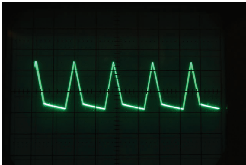
Figure 2. Output waveform, 33 ohm load. Vertical scale: 50 mV/division so the amplitude of the peaks is just over 100 mV. Horizontal scale: 10 \mu s/division, frequency approximately 50 kHz.
