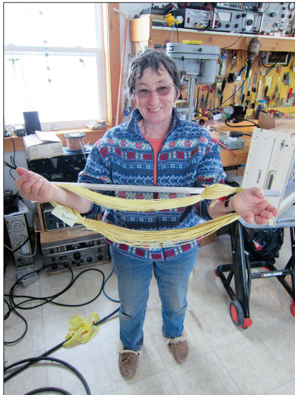
Figure 2: Helen, VA1YL, with 220 feet of Kevlar "boom" and the 41 directors. Total weight 1.6 pounds (730 grams).
