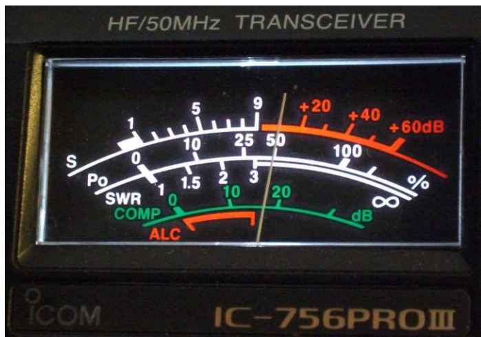
Figure 6: A transceiver multifunction meter showing 50 watts power output (Po).
