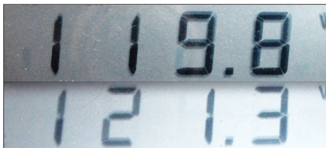
Figure 2: Lower and higher AC mains voltage variations sampled on the same day
