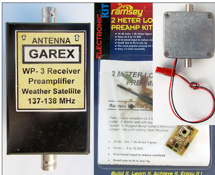
Figure 5: Low Noise Amplifiers. LNAs are available built or as kits you can put inside a metal (for RF shielding) weather and waterproof enclosure.
