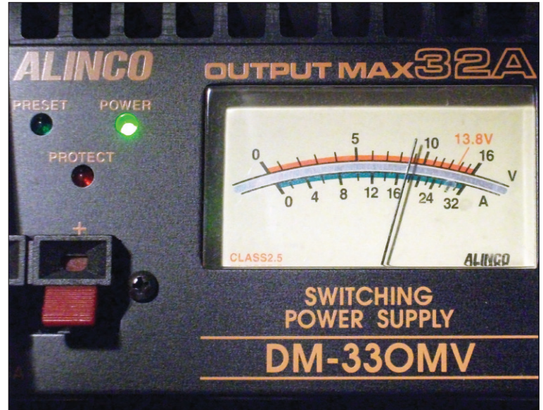
Figure 1: Current draw from the power supply using a built-in meter
